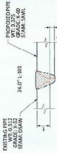
DETAIL 7 WELD (TD-4160P-20) SCALE: NO SCALE
